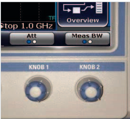
Two rotary knobs with user-assignable functions.
